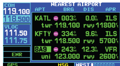
Figure 8-11 Frequency Moved to Standby Field
